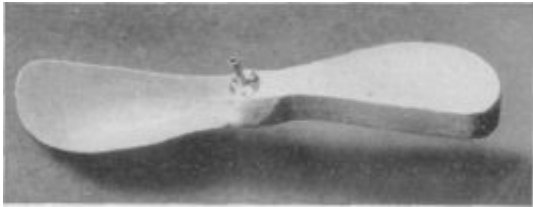
"Finish one end of the blade before cutting away the opposite end"
